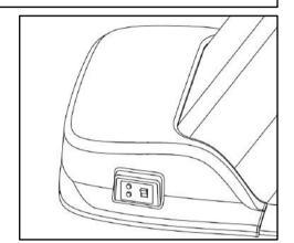
4. Remove the cover and mark the installing position, then move the unit away.
