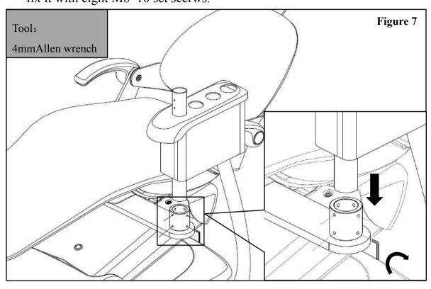
Check the levelness of the water unit through a leveling instrument, change the levelness by adjusting the screws on the post.
