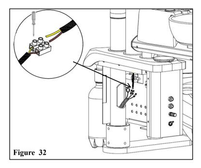
6. Take out the lamp from the package, pass the wire through the cosmetic ring and connect the wire terminals, then joint the light head and the level arm together, fully fasten with a M5\*12 screw.
