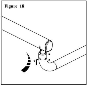
5. Pull out the tubes and wires from the hole of the post, connect the tubes by color and joint the wire terminals.
