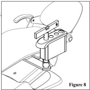
Hold the water bottle upward and align the bottle head gaps to the fixing pins, swivel the bottle clockwise to fix it.
