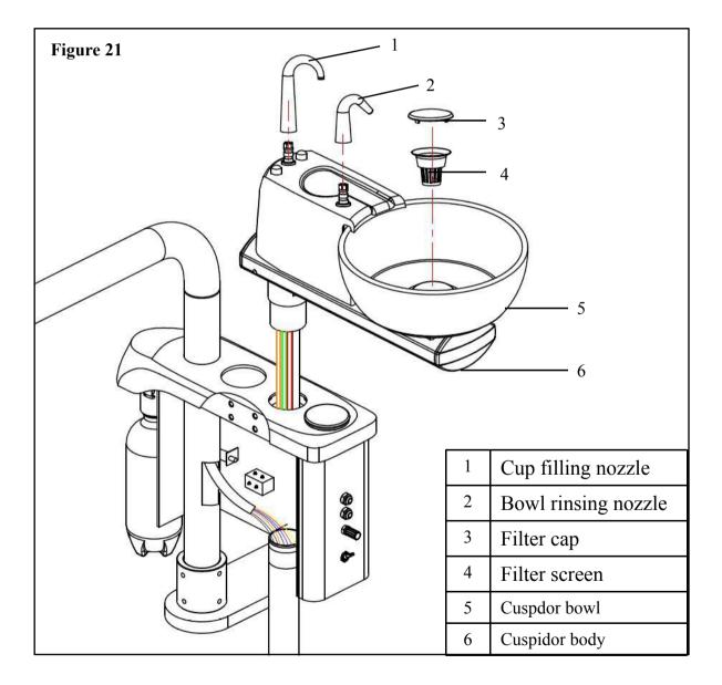
Pass the tubes through the mounting hole and place the connecting shaft into the mounting base.
