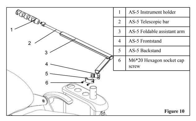
Figure 11 Take out the assistant unit from 1. the carton, loosen the screws counterclockwise to divide the frontstand and backstand so that the arm can be installed on the post of the side box. Tool: 5mm Allen wrench 2. The height of the frontstand and 3. Insert Instrument holder into backstand to the top surface of mounting shaft and lock fastening water unit should be10~20mm; screw. tighten the screw in clockwise. 0-20mm RRARC Figure 13 Figure 12
