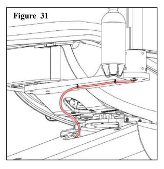
5. Pull out the reserved light wire form the hole, and connect to the light wire from the itermediate post by color.
