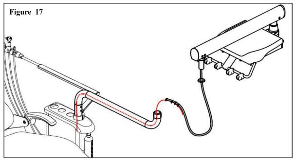
4. Joint the level arm and the rotary arm with three M6\*8 set screws, tighten the screws in clockwise.
