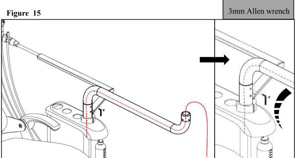
2. Loosen the two screws to remove the cover of the side box, pull out the guide line from the hole of the post.
