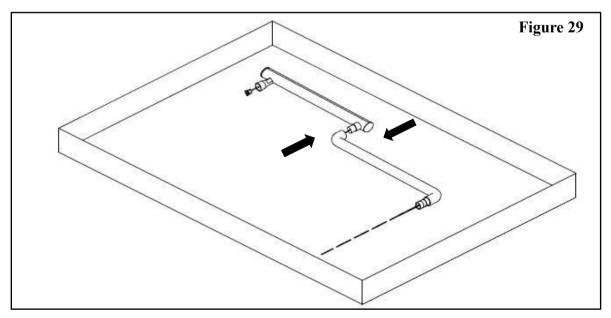
3. Put the connecting shaft of lamp arm into the intermediate post, let the wire pass through the post and reach to the water unit.
