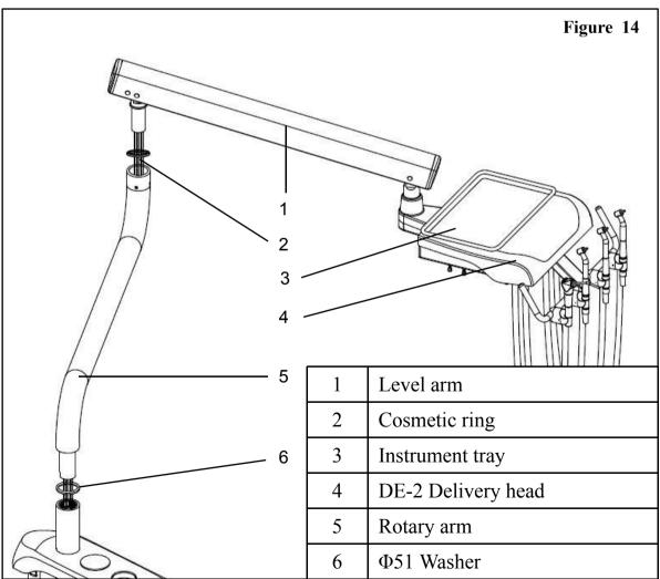
Mount the rotary arm to the post of side box and fix it with two M6\*8 set screws,then insert two M6 plugs. Reserve the guide line.
