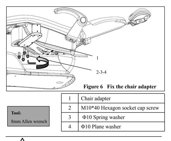
Attention: Completely tighten the screws to avoid
