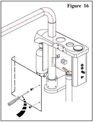
tool: Philip screw driver 3. Let the wire of level arm pass through a cosmetic ring and bind it with the guide line, pull the guide line to route the wire through the rotary arm .
