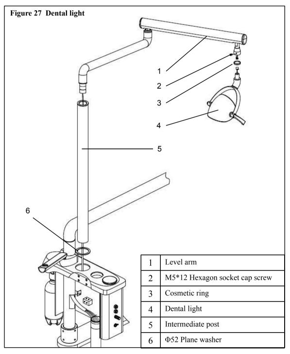
1. Let the intermediate post pass through the plane washer, put the post into the mounting hole and fix the post with M8\*10 set screws.(Move the cover of side box upward can tighten the screws easier.)
