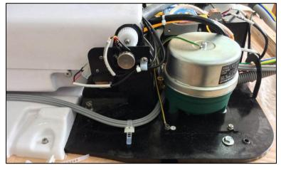
2. Bind the front part of the foot tube and the tube bundle together with zip ties.
