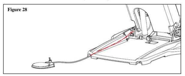
2. Foot control tubes shall bypass the oil can and be tied together with the tube bundle.
