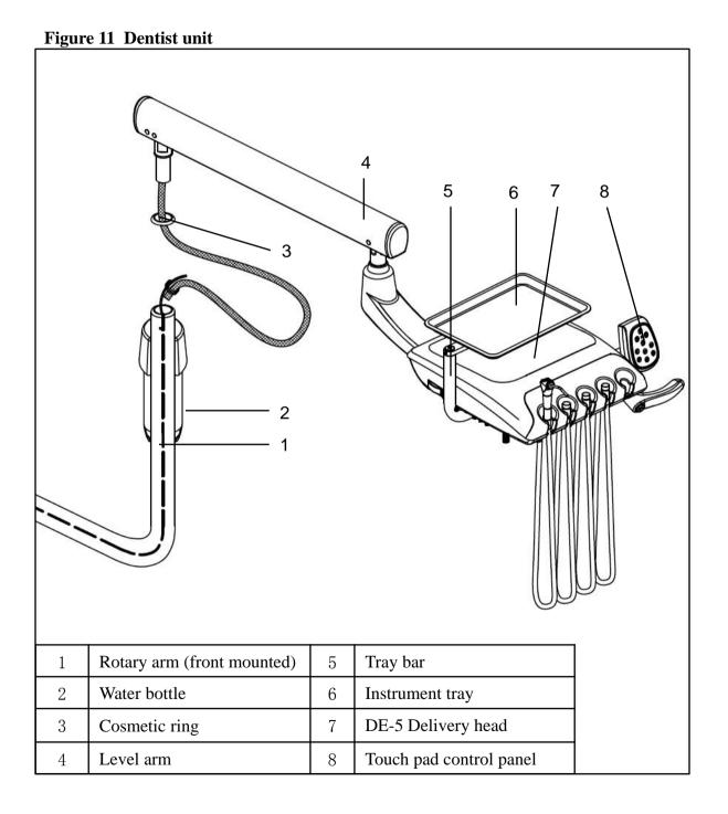
1. Get fixed rotation angle between the bracket of delivery head and the level arm by a M6\*20 screw assembly, in avoid of  $360^{\circ}$  rotation of the delivery head.
