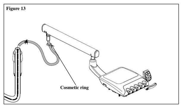
3. Install the unit to the rotary arm, fix it with three M6\*8 set screws and insert the screw caps.
