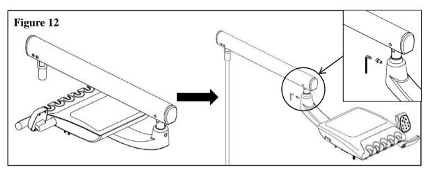
2. Tubes pass through a cosmetic ring and bind with the guide line, pull the guide line to let the wires pass through the rotary arm.
