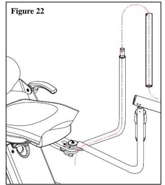
3. Joint the intermediate post and the rotary arm, the jag on the post is screw position .
