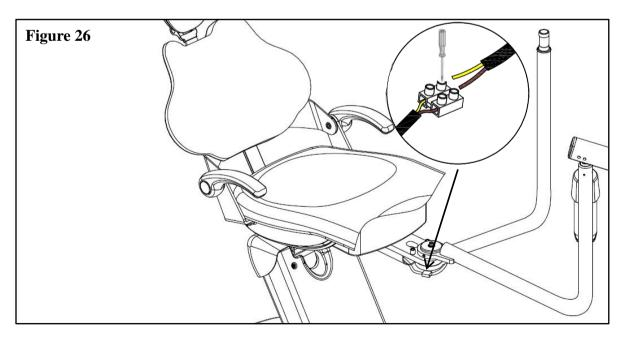
7. Take out the lamp from the package, pass the wire through the cosmetic ring and connect the wire terminals, then joint the light head and the level arm together, fully fasten with a M5\*12 screw.
