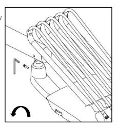
4. Mount fixing tray to the tray holder and lock by threeM3\*10 cuntersunk screws.
