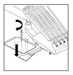
3. Install the tray holder to the bottom of the delivery head and fix it with four M6\*30 screw assemblies.
