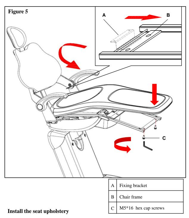
Put the upholstery onto the chair frame, lock the bracket and the rear end of the chair frame together, and tighten the two screws on the front end of the chair frame.
