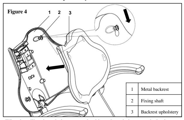
When installing the upholstery, you should put the upholstery on the backrest with the shaft head pass through corresponding keyholes of the upholstery, then push the upholstery in force till it's fixed.
