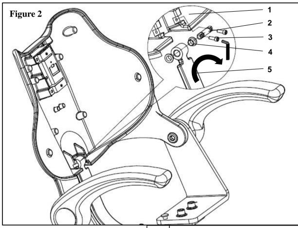
Pass the fixing shaft through the backrest push rod, fix the shaft on backrest with the cap screw assembly.
