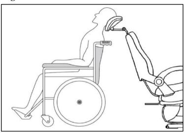
Figure 9 Fix the headrest for a wheelchair.
