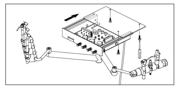
1. Slide and open the top plate, install the unit under the table, fix it with four M6\*25 outer hex Philip's tap screws.
