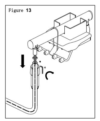
**3**. The tubes of the dentist unit and those reserved of the chair shall be connected by color, and close the cover after connection. Ignore the reserved wires, you have no need to connect them for there's no control panel on delivery head.
