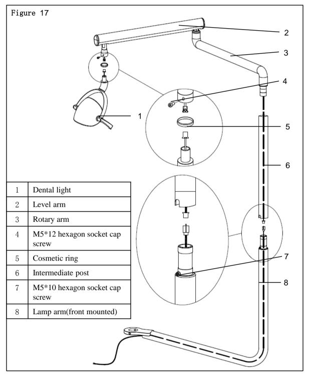
1. Release the M10\*30 screw of the connecting plate, mount the lamp arm to the front mounted connecting plate as the figure shown, then fasten the screw.
