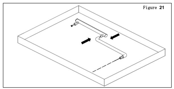
5. Tie the light wire and the guide line together, pull the guide line to lead the wire pass through the post and the lamp arm.
