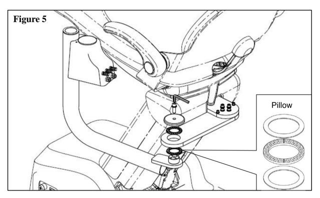
2. Pull the lines of cuspidor from the Rigid arm, insert cuspidor into the Rigid arm.
