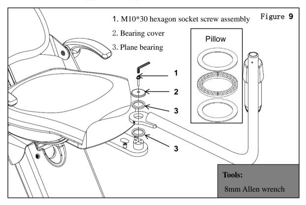
2. Assure the levelness of the rotary by regulating the four screws on the connecting plate.
