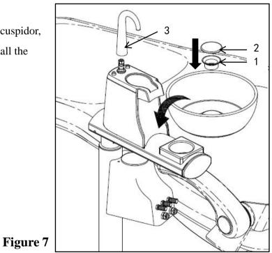
4. Install the assistant hanger under the cuspidor with two screws.
