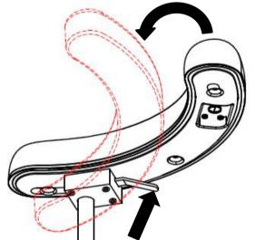
B Push the lever inward and swivel the body support inward, release the lever when get desired position.
