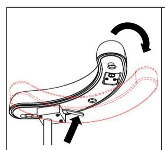
A Push the lever outward and swivel the body support outward, release the lever when get desired position.
