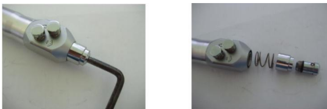
Figure 2 Straight Syringe Tip Locking Retainer Uninstallation
