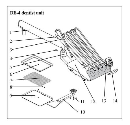
2. Lock the supporting bracket by one M6\*20 screw assembly,to avoid  $360^{\circ}$  swivel of the delivery head .
