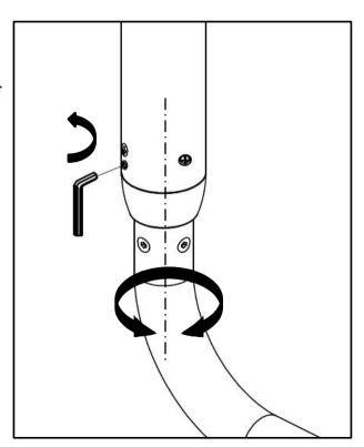
10. Pass the light head shaft through a cosmetic ring and connect the wire terminals, make sure the lamp shaft is well inserted into the level arm, fully fasten with a M5\*12 screw.
