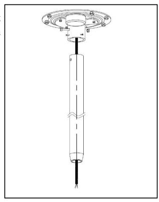
4. Loosen the M8\*90 hex cap screw to insert the light post to the fixing plate, then fasten the nut and four M6\*20 screws to fix the post.
