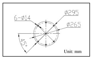
2. Mount the fixing plate to the ceiling with six M10\*90 anchors inserting to the ceiling, and completely fasten the anchors.
